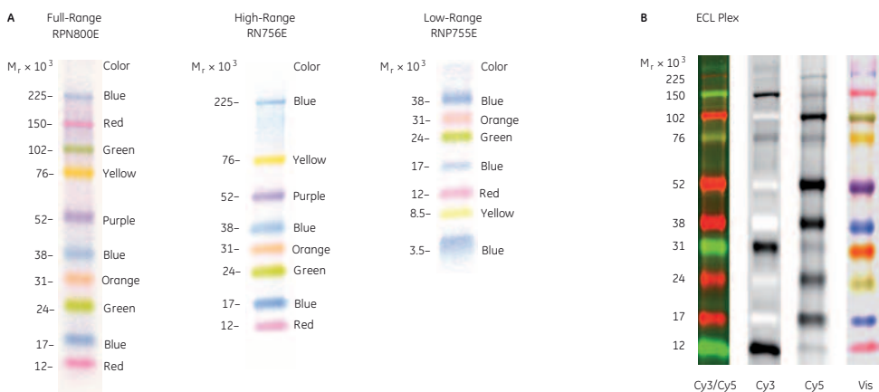
Fig 5.1. (A). Rainbow™ Molecular Weight Markers are available in three size ranges for use with SDS-PAGE. (B). Amersham ECL Plex Fluorescent Rainbow Markers imaged on a Typhoon scanner. From left to right: Full color Cy3 and Cy5, Cy3 channel, Cy5 channel and Visible spectrum.
